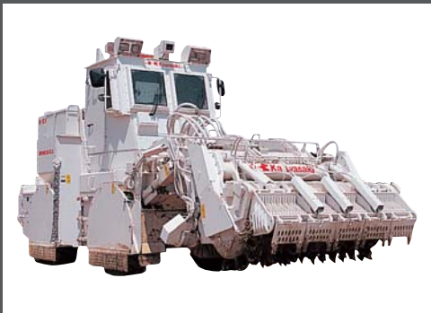
Humanitarian demining system BULLDOG (top: MINEDOG detection vehicle, above: MINEBULL clearance vehicle)
