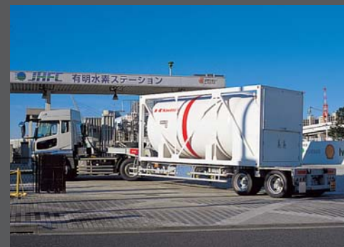
New liquid hydrogen container
